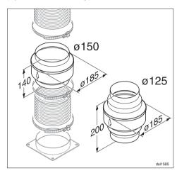
In addition to insulating the exhaust ducting, we recommend that a suitable condensate trap is also installed to collect and evaporate any condensate which may occur. Condensate traps are available for  $\varnothing$  125 mm or  $\varnothing$  150 mm ducting.
